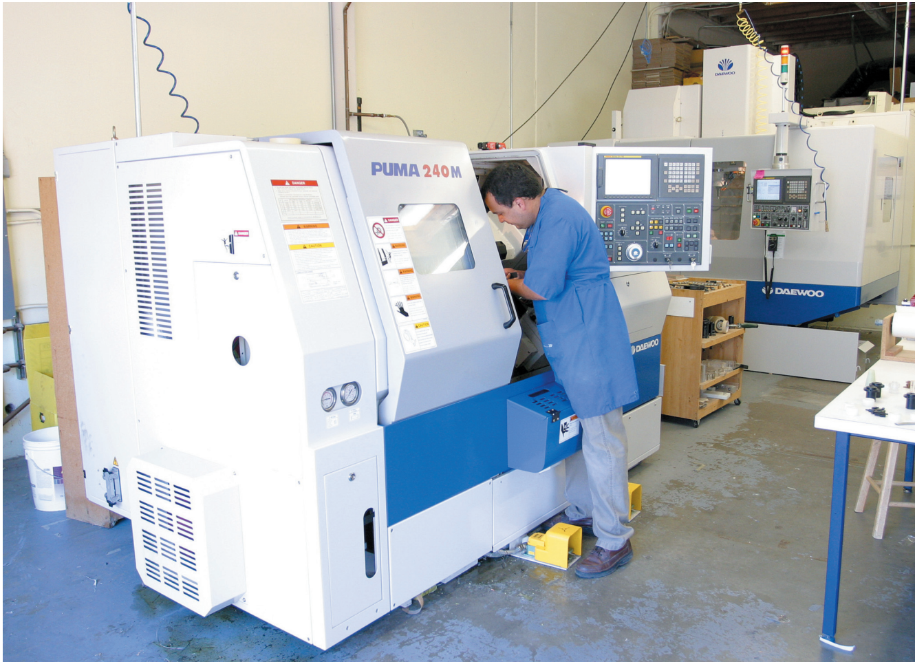
Miguel Rodriguez, CNC Operator, sets up Phoenix Precision Plastic's new Daewoo Puma 240 MA turning center. The machine offers milling, drilling, and tapping capabilities, large bar capacity, high speed spindle, full contouring C-axis, rigid base-mounted tooling (BMT) system, a heavy-duty 12-station turret, 0.1 second turret indexing, one-piece torque-tube slant bed and solid boxway construction. The equipment cruises through the company's plastic machining with ease, according to Donnelly.
