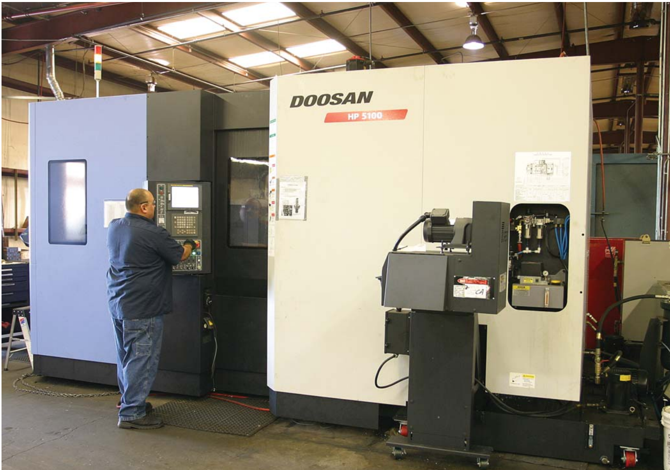
Joe Hernandez, Hydratech machine operator, sets up a recently purchased Doosan Infracore HP-5100 horizontal machining center. The HP 5100 sports a 50-hp spindle motor, dual pallets capable of handling a 1100-lb load, and a 60-tool changer.
