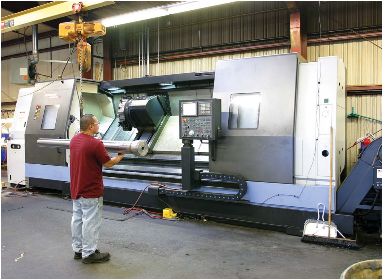
Cho Ly, lathe operator, loads a 15' steel cylinder into Puma 700 CNC Lathe. Cycle time on the 15-ft cylinders is 5 or six minutes, including loading and unloading. The Puma 700 is a true 45° slant bed lathe. The bed is a one-piece casting with both the saddle and tailstock guideways in the same plane to eliminate thermal distortion. A heavily ribbed torque tube design prevents twisting and deformation. The lathe is highly rigid to ensure no deformation during heavy cutting.
