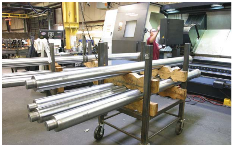
5-1/2" diameter, 15-ft long steel piston rods waiting to be machined on Hydratech's Doosan Puma 700 slant-bed lathe.
